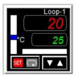
In the Temp, RPM and Pressure Loops you see a 'setting' box (bottom, with green numbers, e.g. 25°C) and an 'actual' box (bottom, with red numbers, e.g. 20°C). In this example, the actual temp is below the set temp, so the white vertical bar has a blue bar within it, indicating the actual temp is below the set temp. If the reactor was heating, a red bar within the white, horizontal bar would appear. Keep an eye on these to be sure your reactor is behaving as you've told it to!
